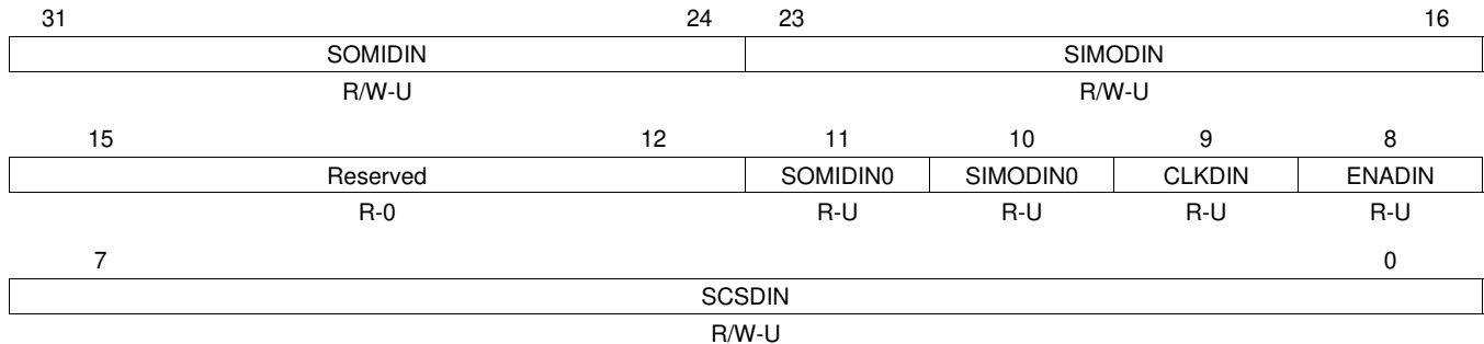
Figure 24-33. SPI Pin Control Register 2 (SPIPC2) [offset = 1Ch]
